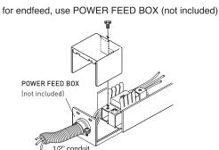
mount FIXTURE HOUSING by using SCREW HOLES at the bottom Step 3
