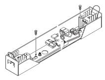
For connecting each fixture, remove the end plate and use I-coupling connector.
